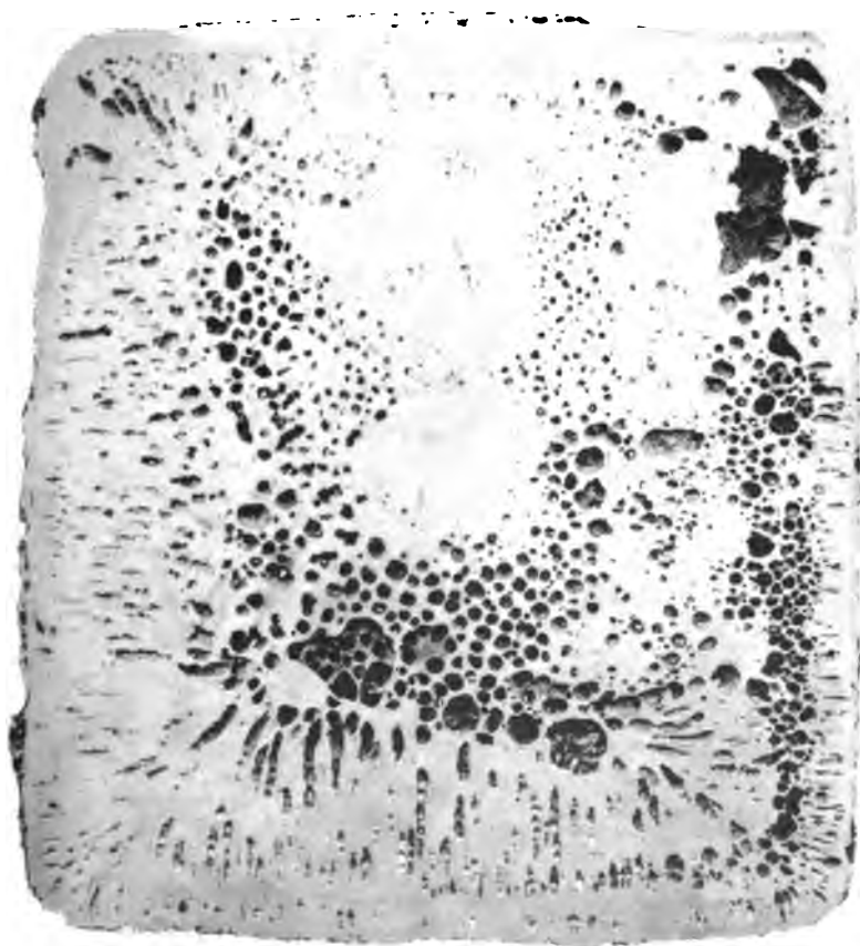
NO. 19. NICKEL STEEL INGOT. BLOCK T1 \frac{1}{2} INCH FROM THE TOP.
